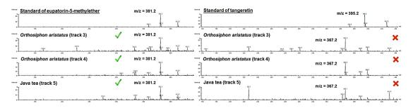
HPTLC-MS spectra of eupatorin-5-methylether and tangeretin and comparison with the corresponding zones in the samples
