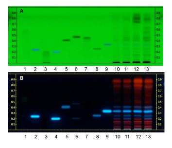
*Revelation under UV 254 nm and UV 366 nm; track 1: rhamnazin; 2: apigenin-4,5,7-trimethylether; 3: 6-methoxyluteolin; 4: luteolin tetramethylether; 5: scutellarein tetramethylether; 6: tangeretin; 7: eupatorin; 8:eupatorin-5-methylether; 9: sinensetin; 10-13: Orthosiphon aristatus*
